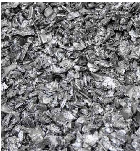
Crushed copper-nickel-aluminum made from condensers.
